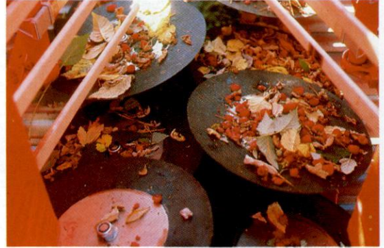
Figure 2. The fruit-catching device of Joonas consists of a rubber tray system.
