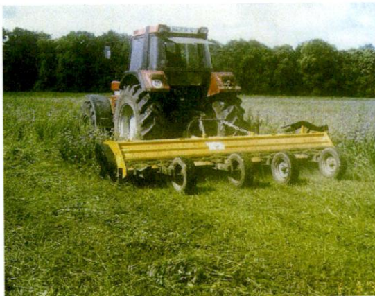
Figure 5: Back mounted flail mulching machine with four supporting wheels (dlz 4/1996, p.79)
