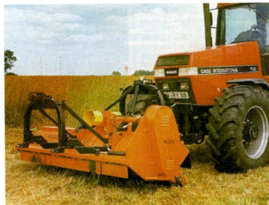
Figure 6: Front mounted flail mulching machine (HASS 1996)
