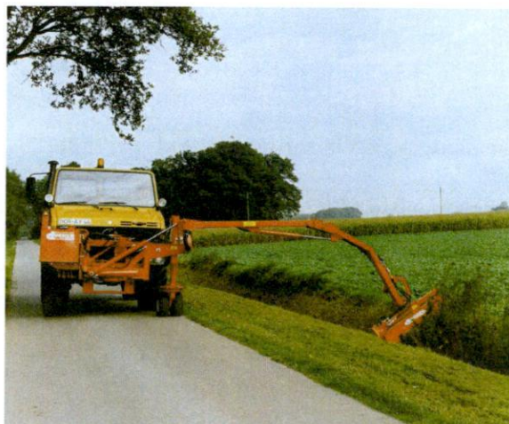
Figure 11: Roadside mulcher (Gerhard Düker KG, Germany)
