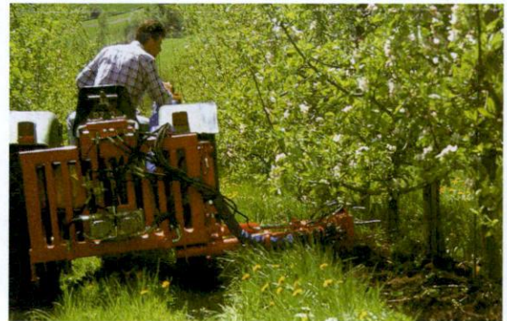
Figure 16: The Ladurner row mulcher works on the right side of the tractor operator (Ladurner Karl J. & Co.-OHG, Italy)
