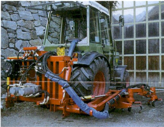
Figure 16: The Ladurner row mulcher works on the right side of the tractor operator (Ladurner Karl J. & Co.-OHG, Italy)
