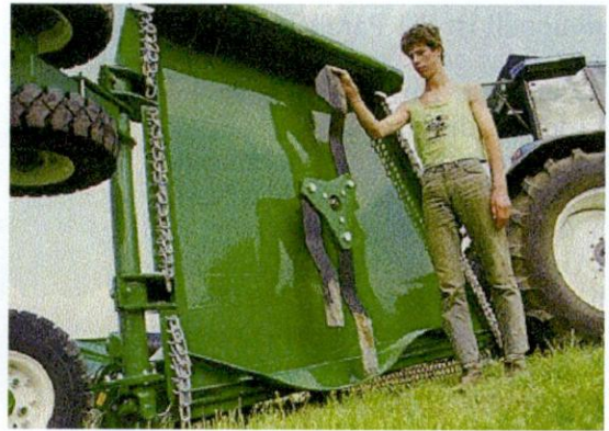
Figure 8: Cutter-assembly of rotary mulching machine (dlz. 2/1997. n.80)
