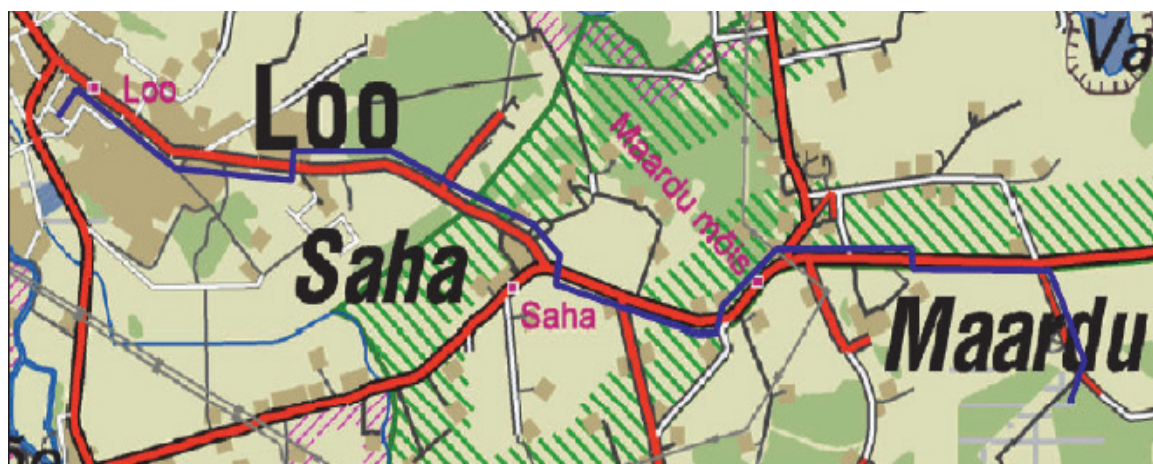
Figure 8. The trajectory of the gas pipeline (marked blue) between the biogas plant in Maardu village and the CHP in Loo settlement (Loo Biogaasijaam ..., 2011)
