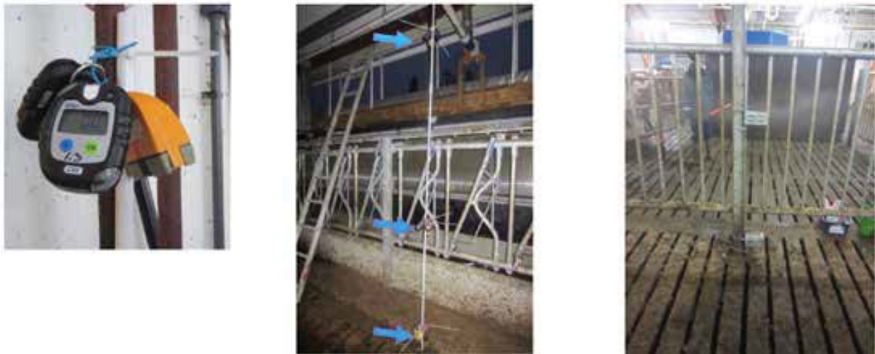
Fig. 1. The Ammonia sensors together with CO 2 , temperature and RH gauges (left) were placed inside the barns in three elevations (0.1, 1.0 and 2.5 meters) (center) and three to four locations, depending on the size of the barn. If accessible to the cows, the instruments were protected by rugged steel casings (right). (Hellstedt & Haapala 2018)
