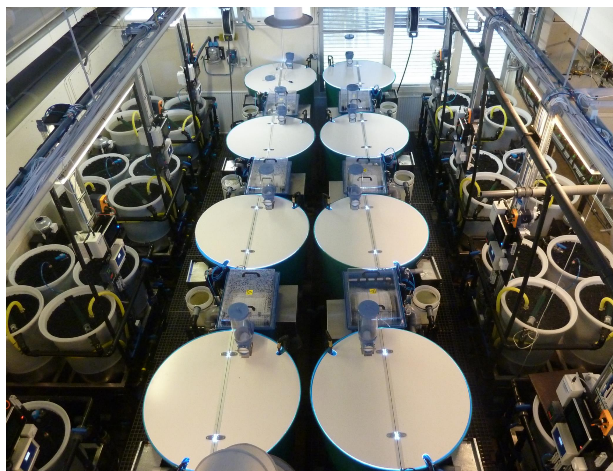
Figure 1. RAS research system used to raise salmonids in central Finland (Photo Tapio Kiuru 14.9.2017).
