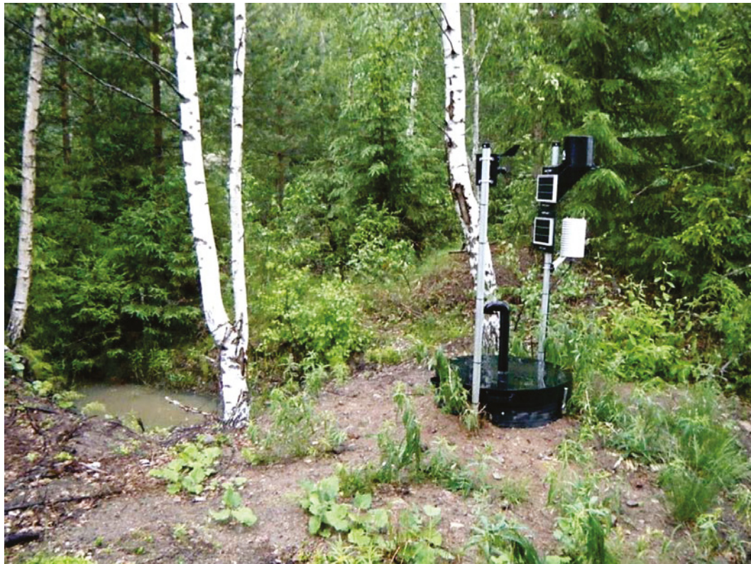
Photo 9. Discharge monitoring station at an outlet of a forest drainage area in Finland. Discharge, turbidity, pH and nitrate concentrations are monitored continuously throughout the year at the station. Photo Sauli Jaakkola.
