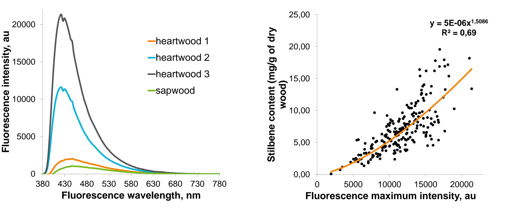
cores was ground for chemical analysis performed with a gas chromatograph. The UV fluorescence measurement was performed on the outer part of the heartwood of the freshly split surface of the other core.
