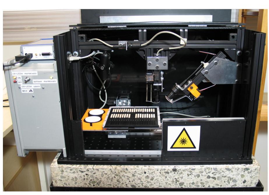
The increment core measurement has been automated with a moving sample plate. Fluorescence is measured step by step for the length of the sample. The measured spectra are corrected with a white reference. An average value for the sample is calculated from the maximum spectral intensity value of each measurement step. A total of
