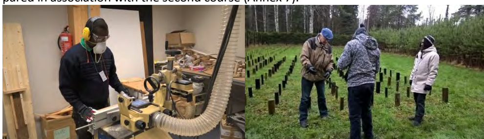
Figure 12. On-the-job training in Finland in November 2015 was focused on the preparation of wood specimens for mechanical analysis and on testing methods of long term durability. (Photos: Veikko Möttönen)
