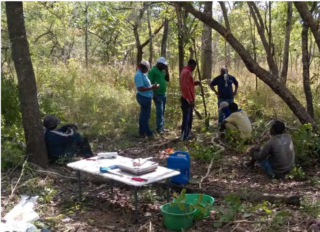
Figure 3. The field measurements of our sample trees included weighing with one scale for max 300 kg with 100 g accuracy (hanging from the tree) and one scale for max 12 kg with 1 g accuracy (on the table). Small sample pieces were submerged into water for volume determination. Photo: Kristian Karlsson.
