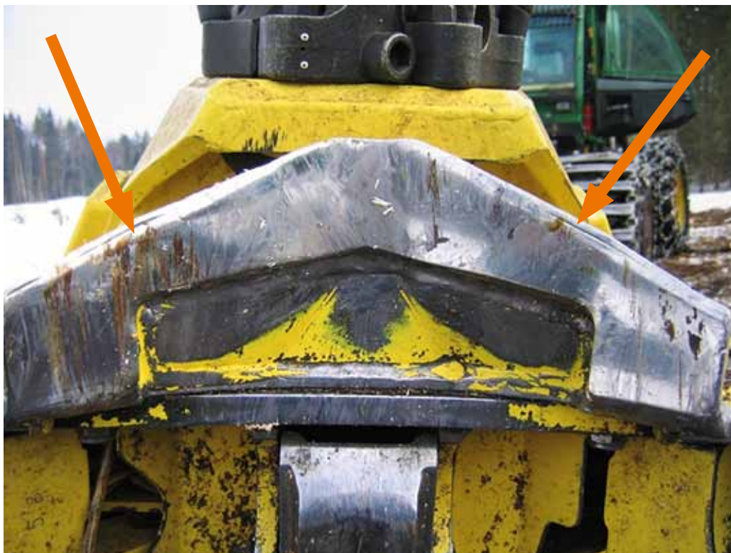
Figure 3.20 Top supporting knife with counter sharpening along the lower cutting edge
