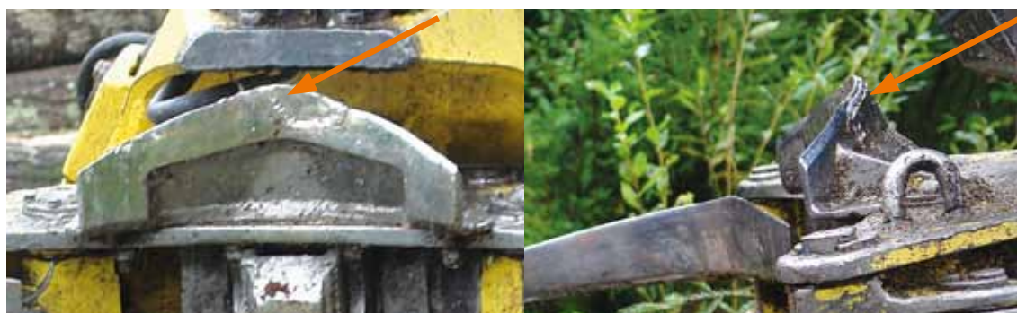
Figure 3.23 Damaged top supporting knife
