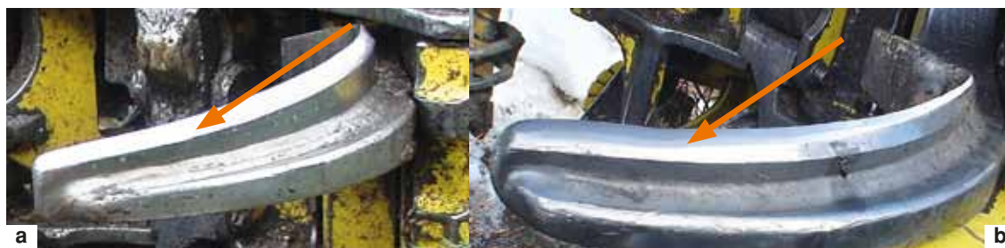
Figure 3.21 Top knife: a – correct angle for cutting branches from thick stems; b – incorrect angle for cutting branches from thick stems
