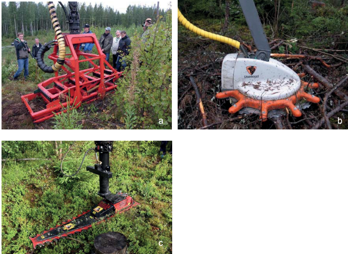
Figure 2. The most commonly used PCT devices in 2015: a) Naarva P25 uprooter, b) UW40 Brushwood Cutter c) MenSe RP6L Hedge Cutter
