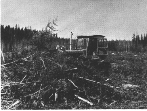
Kuva 5. Oksaraaka-ainetta kasataan Caterpillar D 4-telaketjutraktorilla. Figure 5. Branch raw material is bunched by a Caterpillar D 4 crawler tractor.
