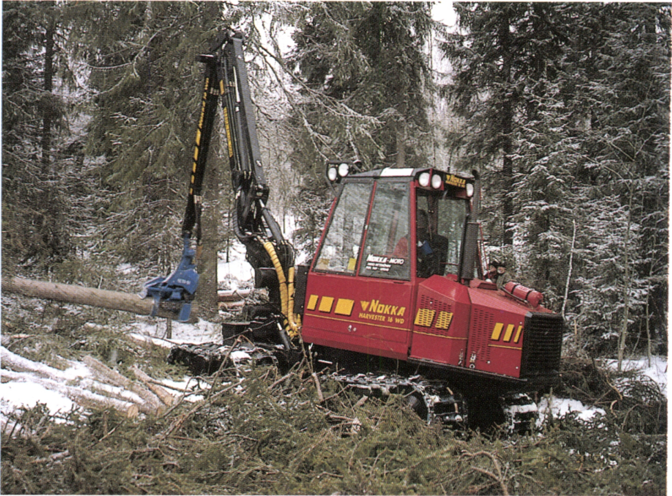
Figure 34. A light tracked one-grip harvester for thinning cuttings. Nokka 16WD equipped with Keto 51 harvester head (Photo Tume Oy).
