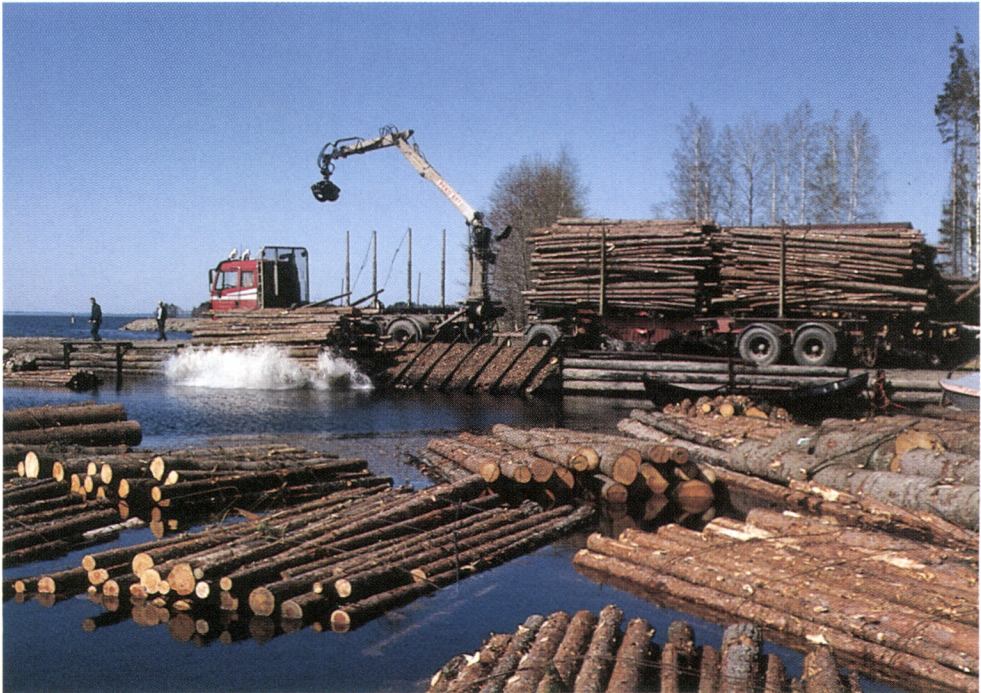
Figure 25. At long distances, road transport is often supplemented with bundle floating (Photo Hannu Kalaja).
