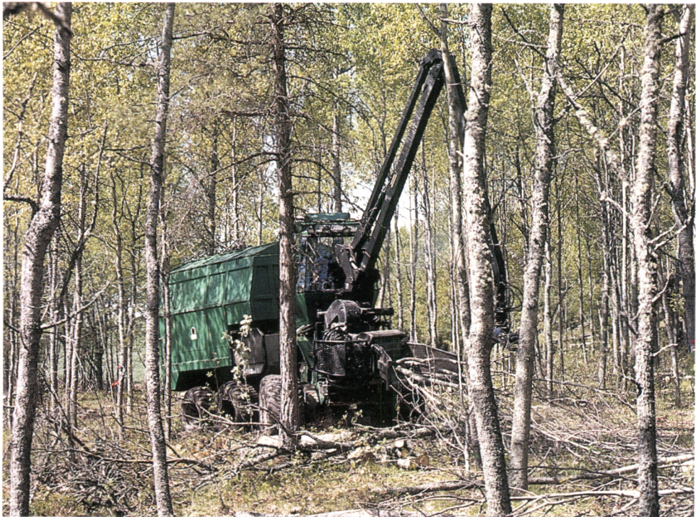
Figure 33. A new mobile whole-tree chipper for thinning conditions. Feeding from both sides and front of the unit. Chipset chipper (Photo Pentti Hakkila).
