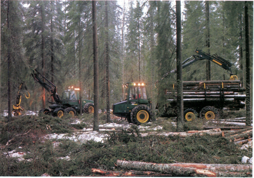
Figure 13. Mechanized cutting and off-road transport are combined into one logging contract and performed with a single-grip harvester and forwarder. Timberjack 1270 harvester and Timberjack 1010 forwarder (Photo Timberjack Europe).
