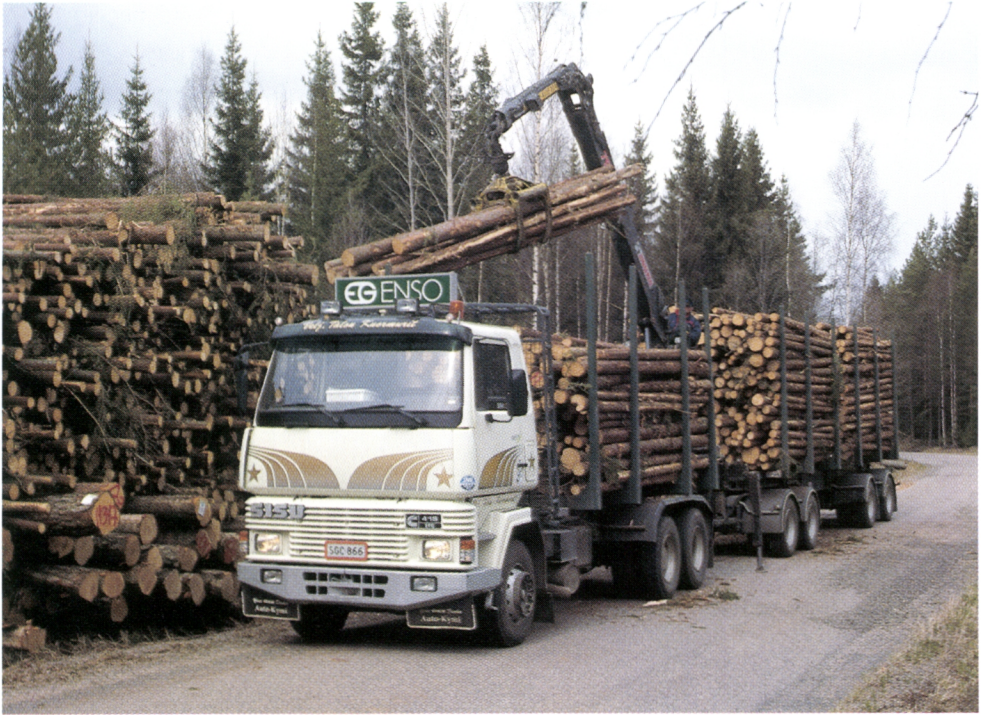
Figure 24. A seven-axle timber truck unit loading spruce pulpwood. Sisu SM 312 truck (Photo Erkki Oksanen).
