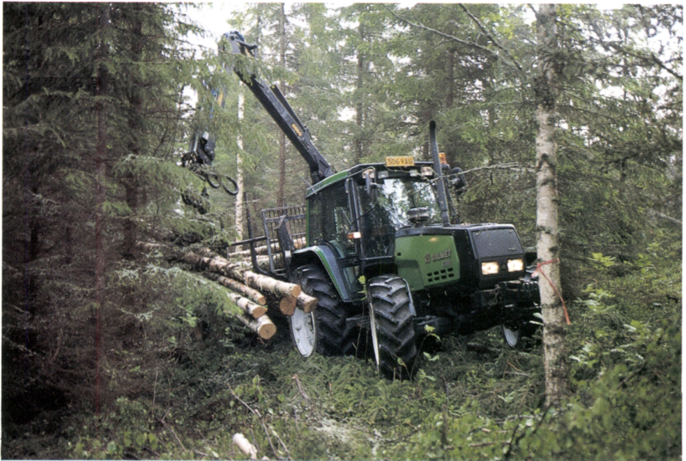
Figure 14. Farm tractor equipped with a hydraulic crane and trailer is a common solution for off-road transport of timber in delivery sales from private forests. Valmet 6300 farm tractor, Kronos 5000 crane and Hakki-Souvari trailer (Photo Hannu Kalaja).
