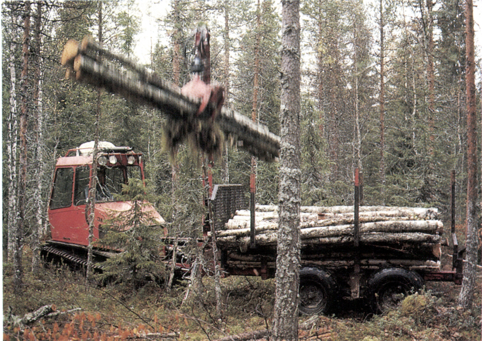
Figure 10. Harvesting small-sized timber from drained peatlands requires special equipment. Forwarding with a light rubber-tracked Fami-Trac crawler (Photo Hannu Kalaja).
