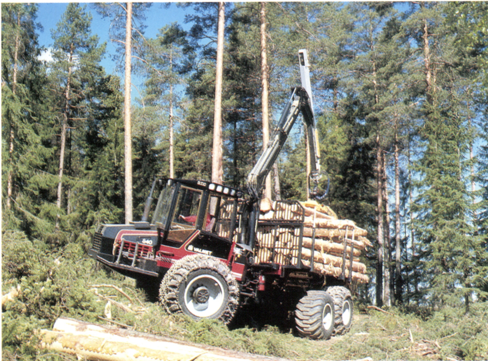
Figure 23. A forwarder hauling sawlogs. Six-wheeled Valmet 840 (Photo Sisu Logging Oy).
