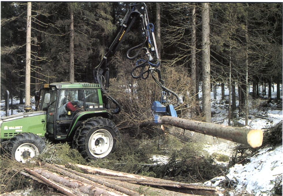
Figure 16. Valmet 6600 farm tractor equipped with Keto 51 one-grip harvester head (Photo Erkki Oksanen).
