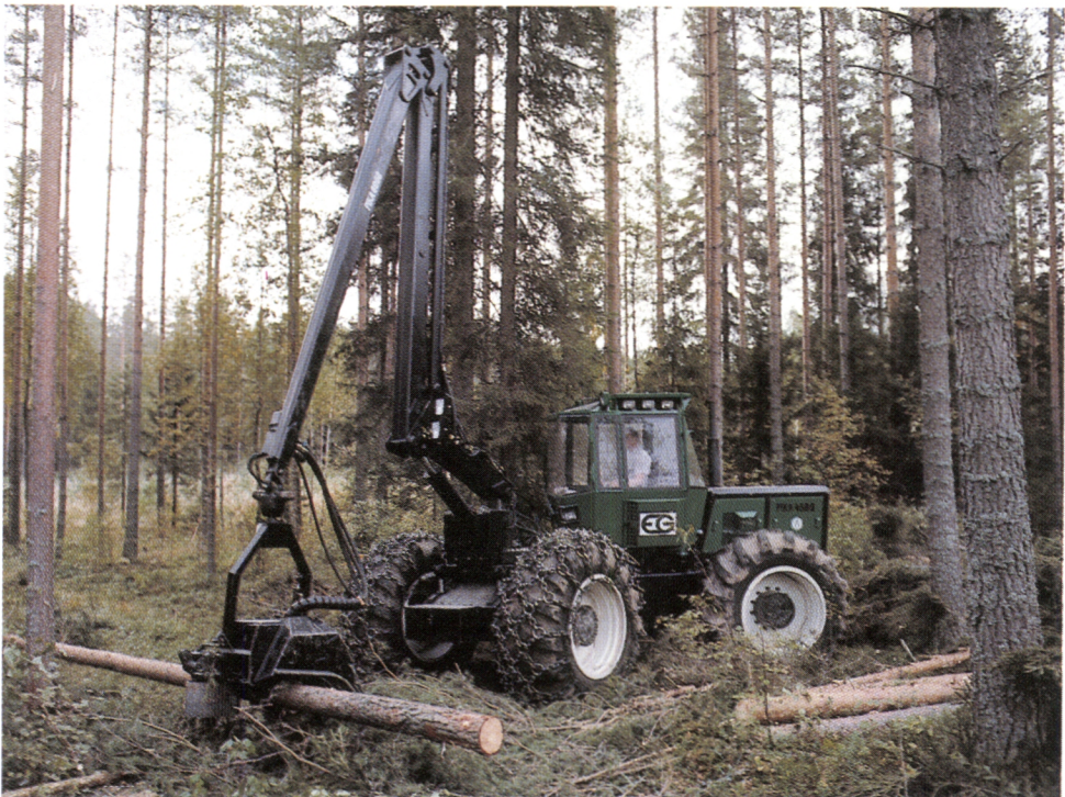
Figure 35. A four-wheeled one-grip harvester. PIKA 4500 (Photo S. Pinomäki Ky).
