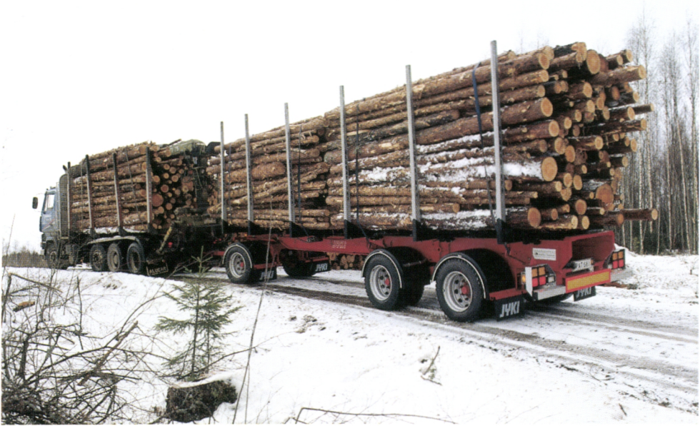
Figure 27. Timber trailers can accommodate two bundles of 6-m logs in tandem. Three-axle Jyki trailer with an extendible frame (Photo Jyki Oy).
