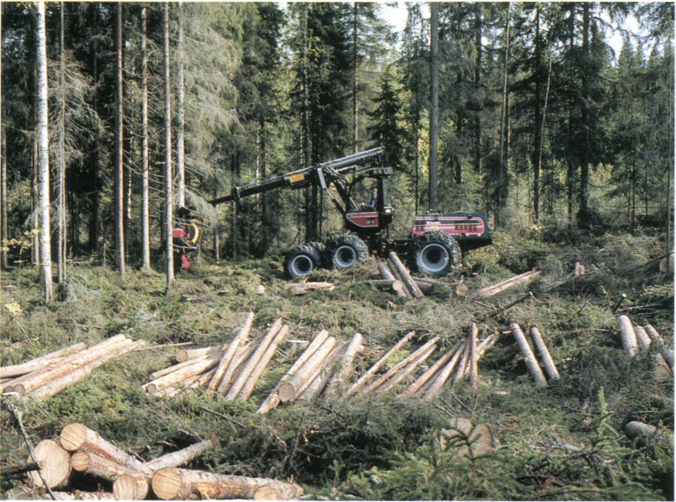
Figure 18. A one-grip harvester clear-cutting a spruce stand for regeneration. Valmet 911 (Photo Sisu Logging Oy).
