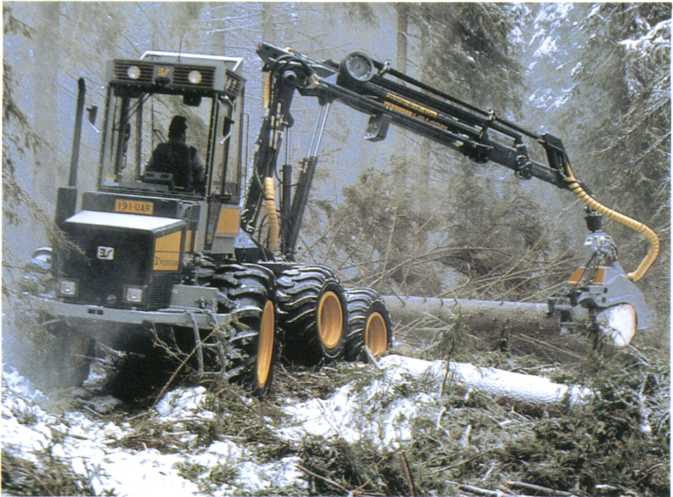
Figure 19. A one-grip harvester processing and simultaneously volume scaling a spruce stem. Ponsse HS 15 Ergo (Photo Ponsse Oy).
