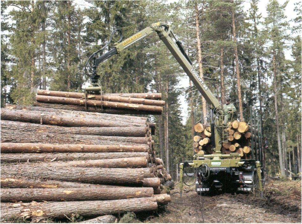
Figure 26. To reduce landing area requirements and for flexible mobility from site to site, timber trucks are self-loading. Loglift 95 timber crane (Photo Loglift Oy Ab).
