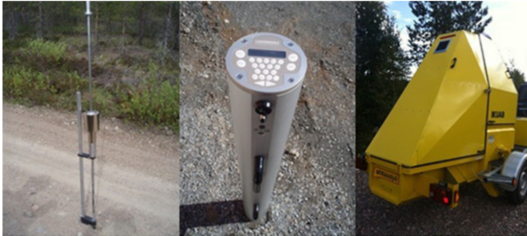
Fig. 3. Test devices, dynamic penetrometer (DCP), Loadman (LFWD) and falling weight deflectometer (FWD).
