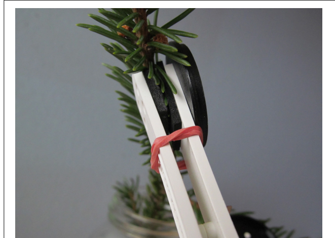
FIGURE 1 | Clips used to measure chlorophyll fluorescence modified with an extra foam pad added to the lower jaw and a small rubber band to draw the clip closed. These modifications helped provide a light-proof closure of the clip around the needles to be measured.
