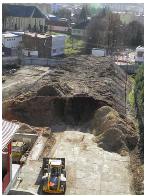
Figure 34. Place for storage of biomass close to the heating plant in Hriňová (Source: Otepka, 2013).
