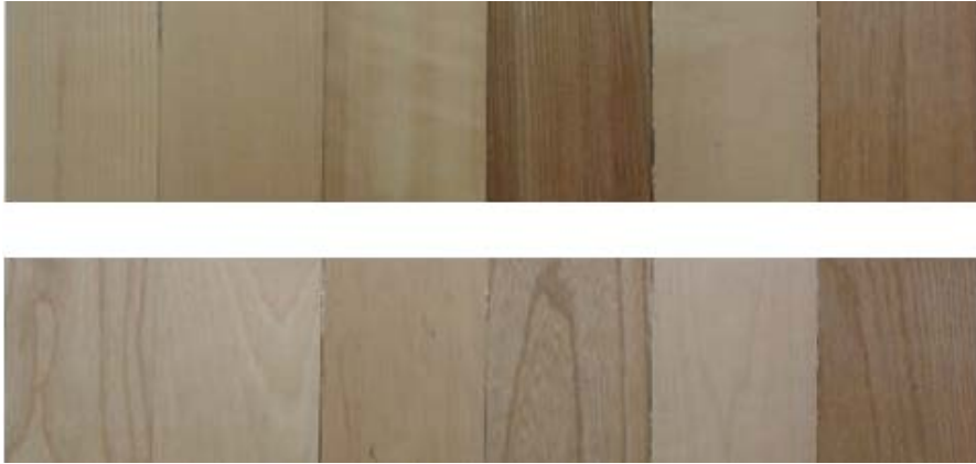
Figure 1. Radially sawn (top) and flat-sawn hardwood boards used in moisture buffering test. Species from left: ash, birch, black alder, elm, maple and oak.
