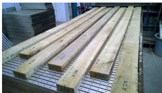
Figure 1. (Left) A set of aspen boards (40 × 100 × 2,700 mm 3 ) before the modification. Photo: Nextimber Ltd.
