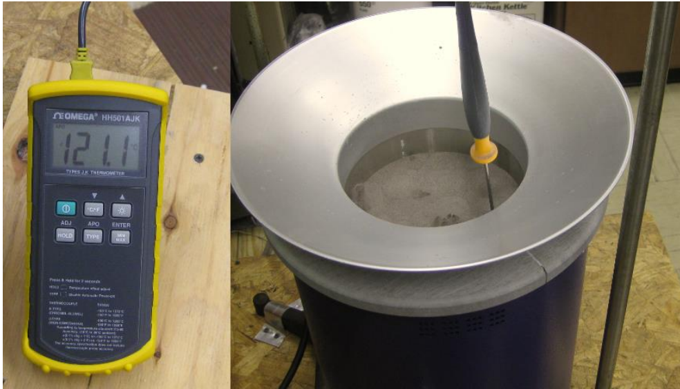
Figure 2. Reaction temperature of sand bath controller
