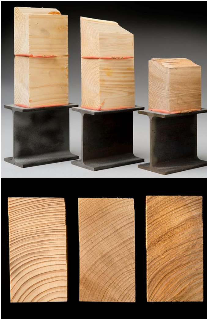
Figure 3. Typical failure modes in tension (above) and compression (below). From left to right: spruce (t), spruce (t), ash (t), spruce (c), beech (c), ash (c).
