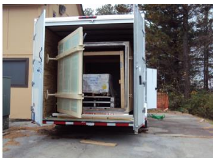
Figure 4. Photograph of vacuum steam chamber used in the tests.
