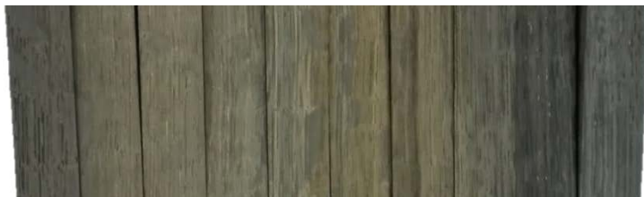
Figure 3. Color difference from the central to the outer part of the plank
