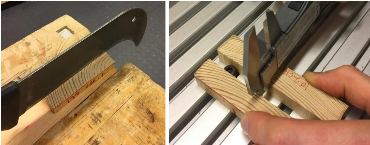
Figure 3. (Left) Method to split the specimens. Photo: Barnes Owusu Sarpong.
