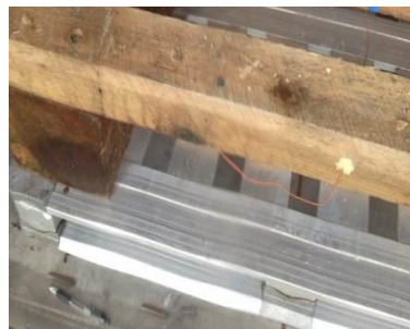
Figure 3. The locations in the large timber of temperature probes and larvae.
