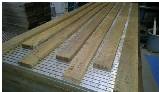
Figure 1. (Left) A set of aspen boards (40 × 100 × 2,700 mm 3 ) before the modification. Photo: Nextimber Ltd.
