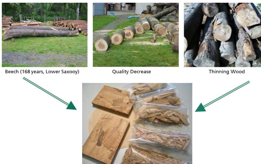
Figure 1. Processing of beech wood assortments to OSB
