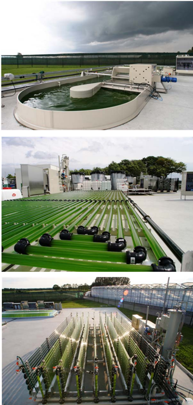
Figure 1. Outdoor cultivation systems (from top to down: raceway pond, horizontal tubular and vertical tubular) in operation at AlgaePARC facility, in the Netherlands. (Photos by courtesy of Dr. Rouke Bosma at Wageningen UR, AlgaePARC).
