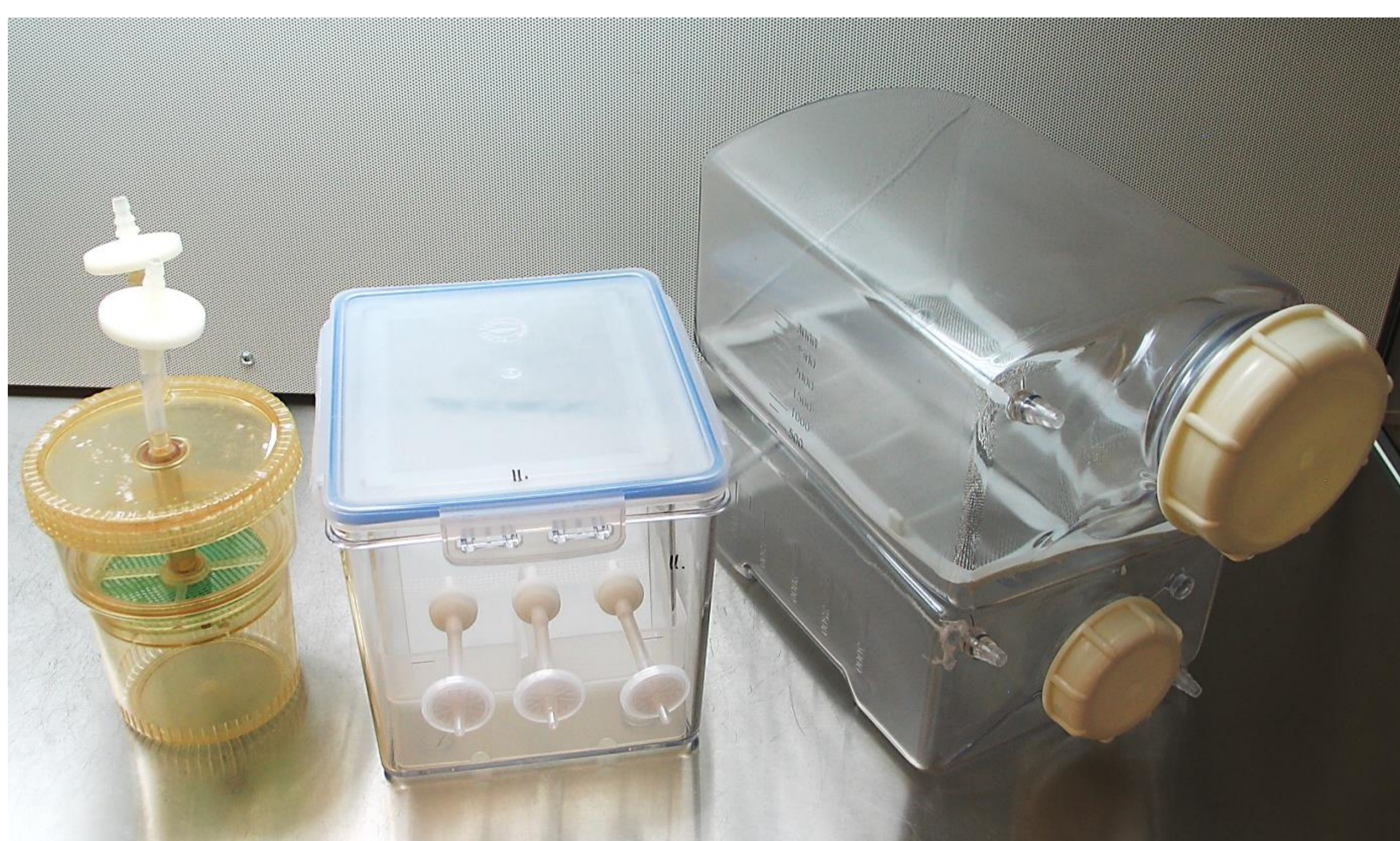
Fig.1 Example of commercially available TIS models. From left to right: Rita®, Plant Form and SETIS™.
