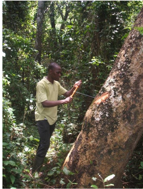
Figure 4: Collection of wood samples using an increment borer.
