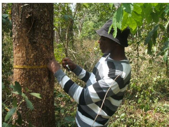
Figure 1: Stem diameter measurement using a diameter tape
