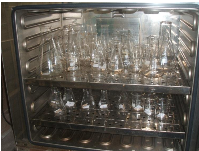
Figure 5 : Wood samples oven-dried at 75 °C to a constant weight
