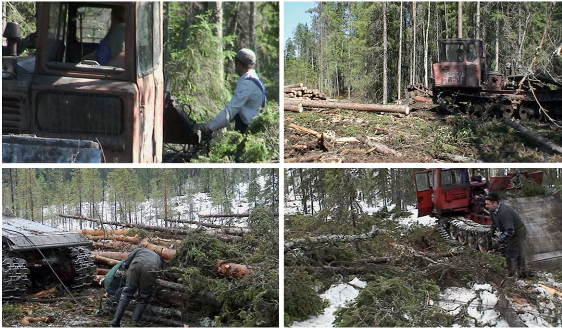
Fig. 4.27. Uncomfortable body positions during operations with a cable skidder
