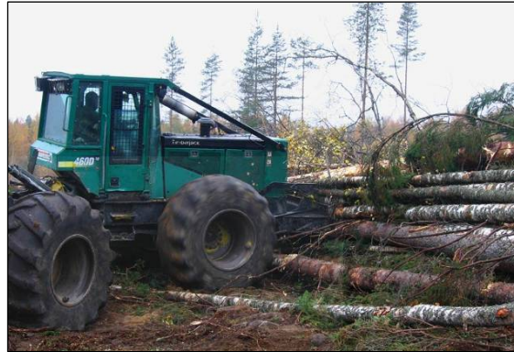
Fig. 5.25. Incorrect piling operation
