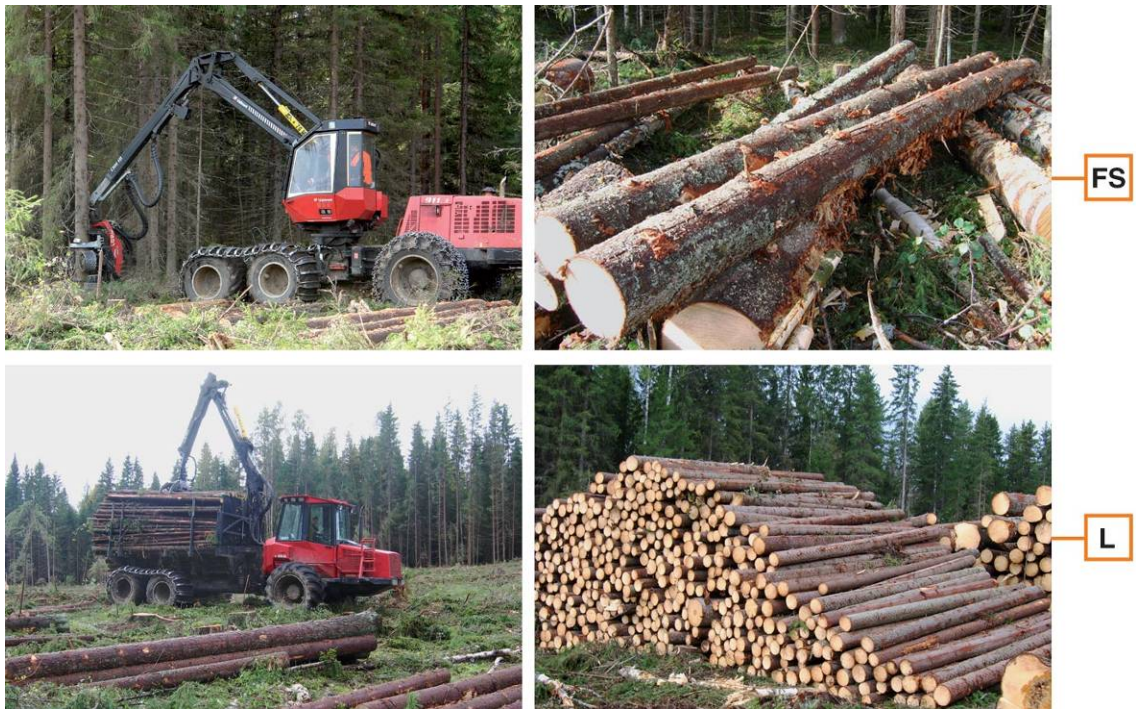
Fig. 5.2. Measurement of logs in fully mechanized cut-to-length harvesting (harvester + forwarder): FS – at the felling site, L – at the upper landing
