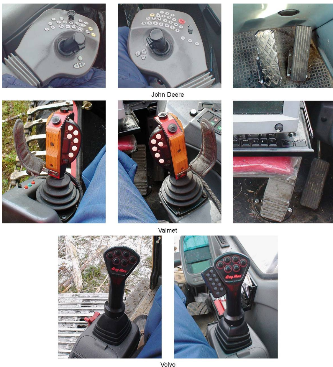
Fig. 4.7. Main harvester controls
