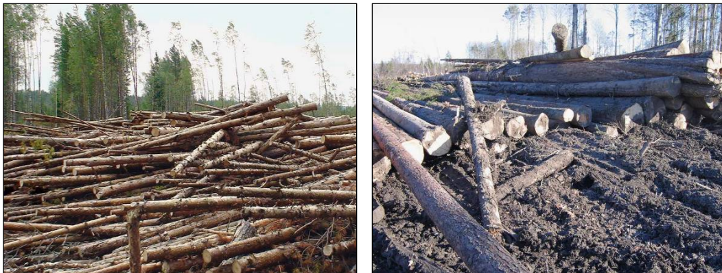
Fig. 5.26. A roundwood pile at the upper landing (loading site) without underlying bed logs
