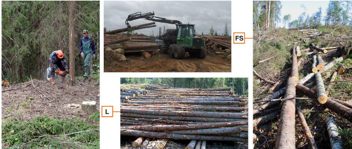
Fig. 5.1. Measurement of logs in partially mechanized cut-to-length harvesting (chainsaw + forwarder): FS – at the felling site, L – at the upper landing
