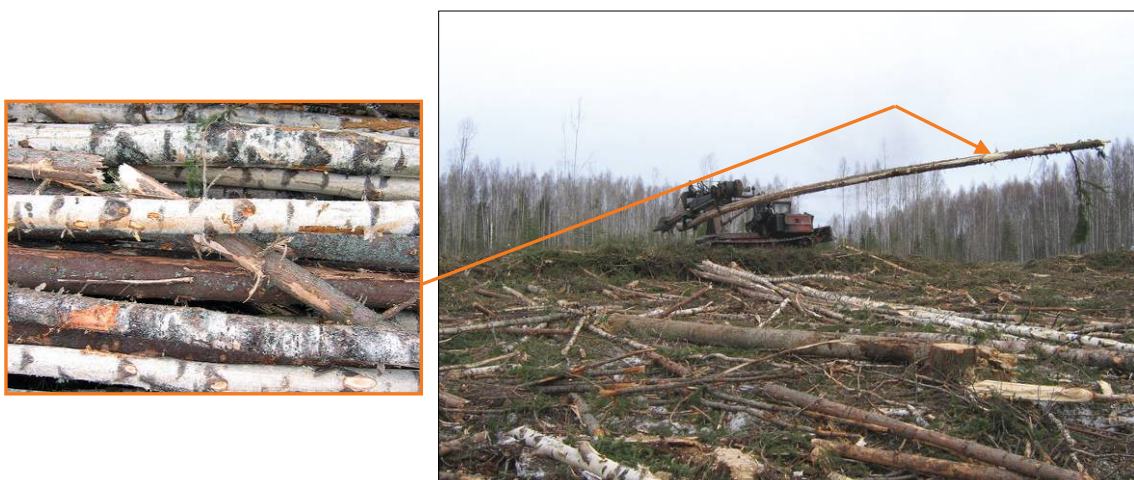
Fig. 5.20. Improper operations during delimiting
