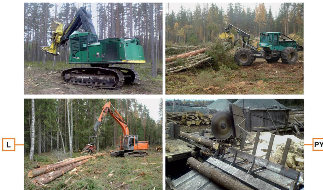
Fig. 5.5. Measurements during fully mechanized full-tree harvesting (feller buncher + skidder): L – tree-lengths at the upper landing, PY – logs at the central processing yard
