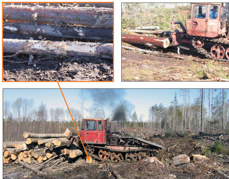
Fig. 5.19. Improper operations during piling of tree-lengths
