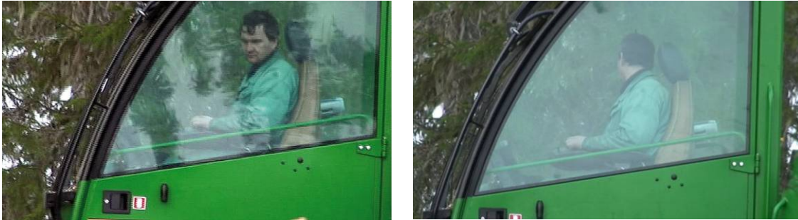
Fig. 4.5. Uncomfortable body positions when operating a harvester without a rotating cabin
