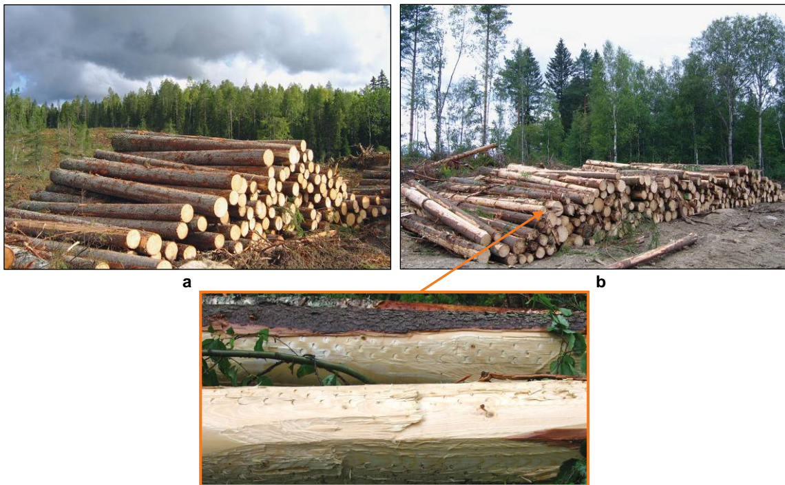
Fig. 5.23. Logs harvested with correctly (a) and incorrectly (b) adjusted harvester head.
