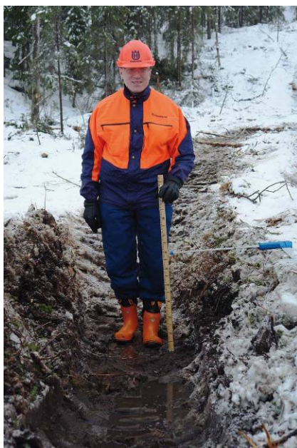
Fig. 3.2. Measurement of trail depth
