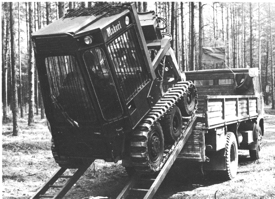
Figure 2. The Makeri tractor can be transported on a light truck.
