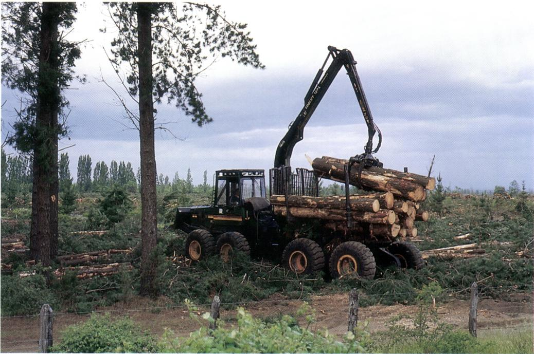
Figura 15. Tractor autocargable Timberjack 933F. *Figure 15. Timberjack 933F forwarder.*
