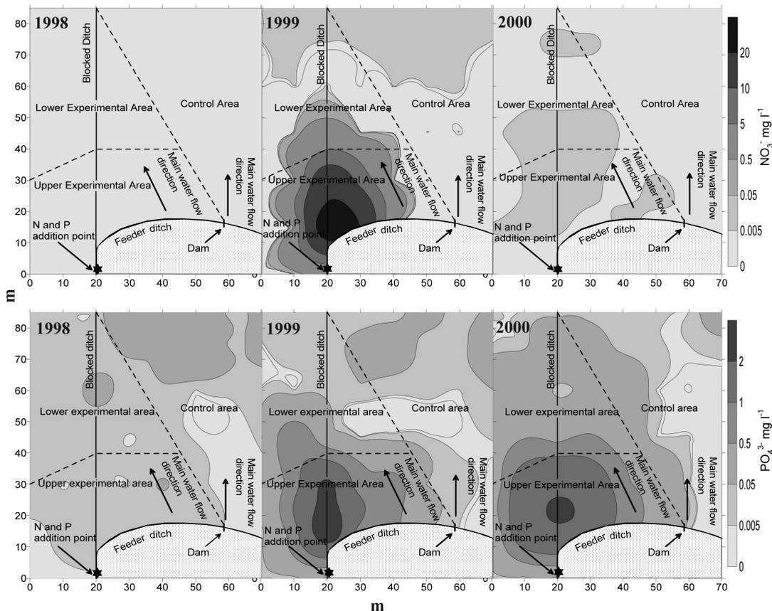
**Fig. 4.** Spatial variation in  $\text{NO}_3\text{-N}$  and  $\text{PO}_4\text{-P}$  concentrations ( $\text{mg l}^{-1}$ ) in soil water in the restored peatland buffer during 1998–2000. The average  $\text{NO}_3\text{-N}$  and  $\text{PO}_4\text{-P}$  concentration values for the summer of each year were calculated from water samples taken 3–4 times during the period.
