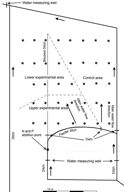
**Fig. 1.** Schematic map of the site, showing the N and P addition point, feeder ditch, and main water flow directions. Filled circles are water sampling wells.
