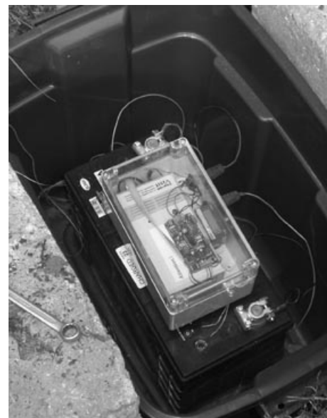
Figure 3. VisitLog and battery in a plastic-box lined.
