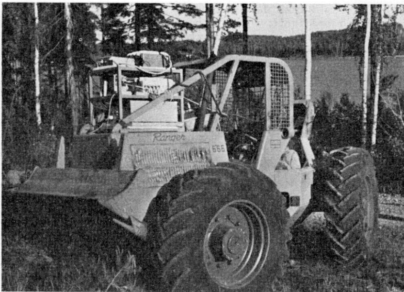
Figure 4. The amplifying- and register equipments of the measurement signals, on a skidder.
